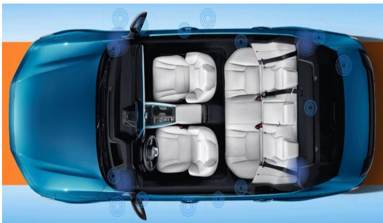
Active noise reduction system, new three-axis vibration sensor, high-precision detection of tire noise, audio pronunciation to offset noise
